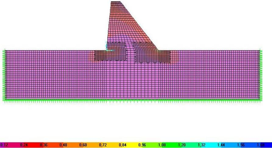
Figure (7) Envelope Maximum Stress (S11) (static loads condition).
