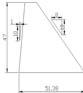
Figure (1): Geometric configuration for Mujib dam
