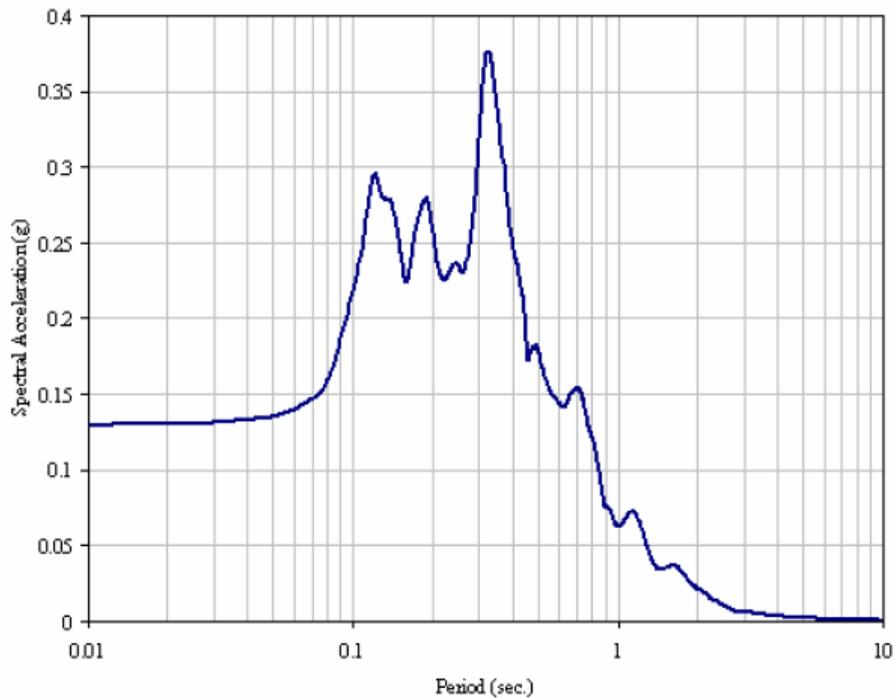
Figure (4): OBE Response Spectra for 10% Damping
