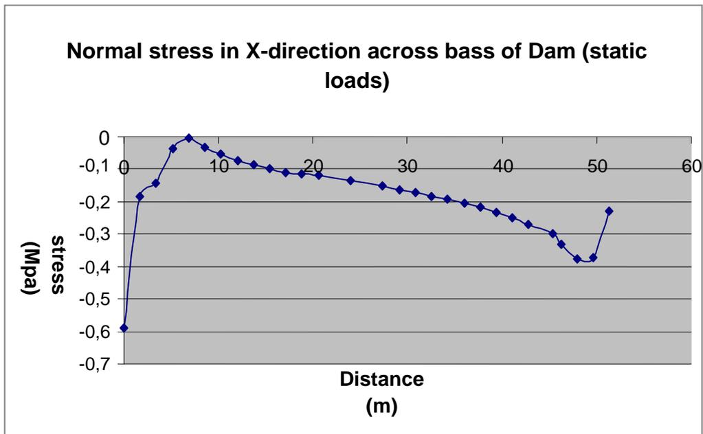
Figure (10): Normal stress in X-direction across Bass of Dam (Static Case).
